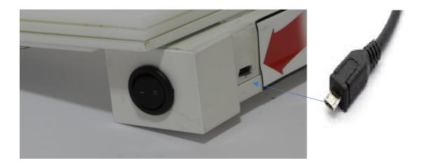
The device is charged with the mobile phone charger power of 5V which is limited to 700 mA. The connection for the charging is micro USB jack.
